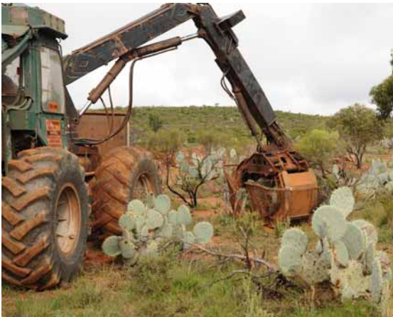
Mechanical control using a grapple arm to 'pluck' Opuntia robusta (wheel cactus) from the ground
