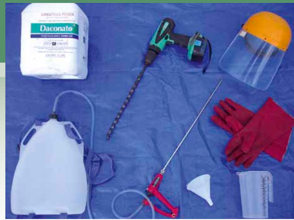
Equipment for stem injection, including Daconate herbicide, stem injection kit, drill, plastic gloves and face shield
