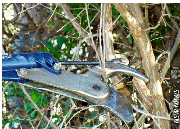
The blade of the pneumatic shears; the shears are run from an air compressor based on a trailer
