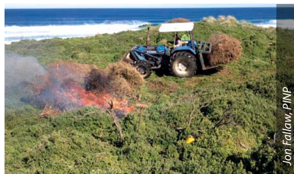
The tractor used on Phillip Island, adapted to grab the uprooted boxthorn and place it on piles for burning
