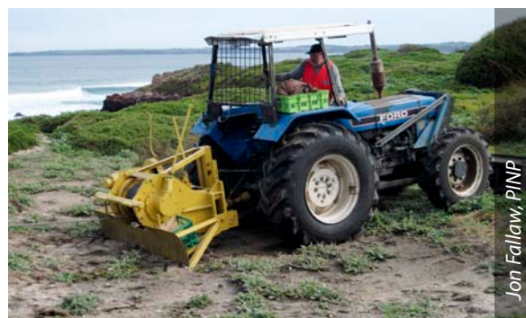
On Phillip Island, a winch on the back of the tractor pulls boxthorn out of the ground by putting a chain noose around the stump and winching it out
